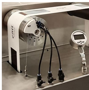
Sealing segment for actuating and tool-free verifying of the contact angle and width
